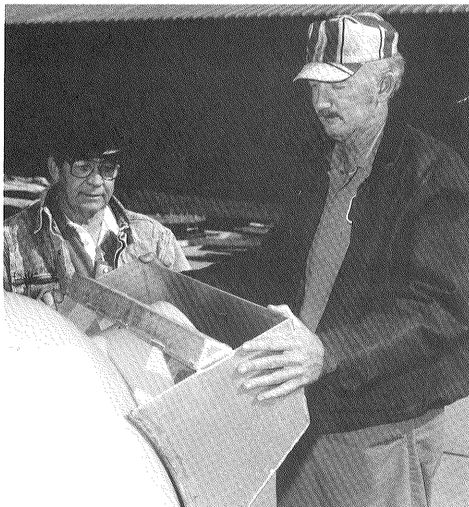
Jim Arthur and Jim Hull look over the device they designed and fabricated to serve as a reservoir for dry ice around valves of 10-ton and 14-ton product cylinders. The pans allow dry ice to be quickly and securely contained around the valve, cooling the valve and valve area of the cylinder, solidifying the uranium hexafluoride and stopping a leak.
